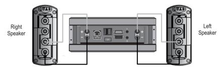
Choose a suitable length of twin core speaker cable for each channel, and prepare the ends as described above.
