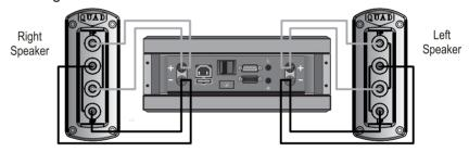
Most of the audio signal going to the speakers drives the bass units. Where one cable feeds both bass and treble units, this heavy bass current can modulate the high frequencies. Using separate cables for treble and bass units reduces intermodulation effects and improves headroom and clarity. This technique of wiring is known as Bi-Wiring. To bi-wire, you will need to install two lengths of twin core cable between the amplifier and each loudspeaker.
