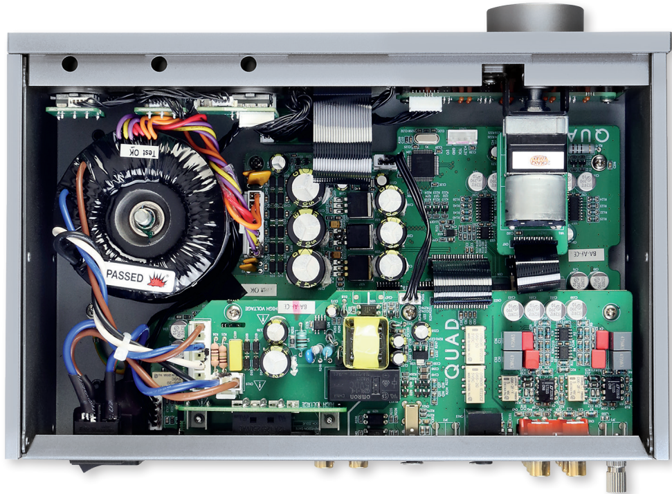
Every inch the modern preamp – Quad's 33 features a motorised volume control and switchmode PSU for standby
